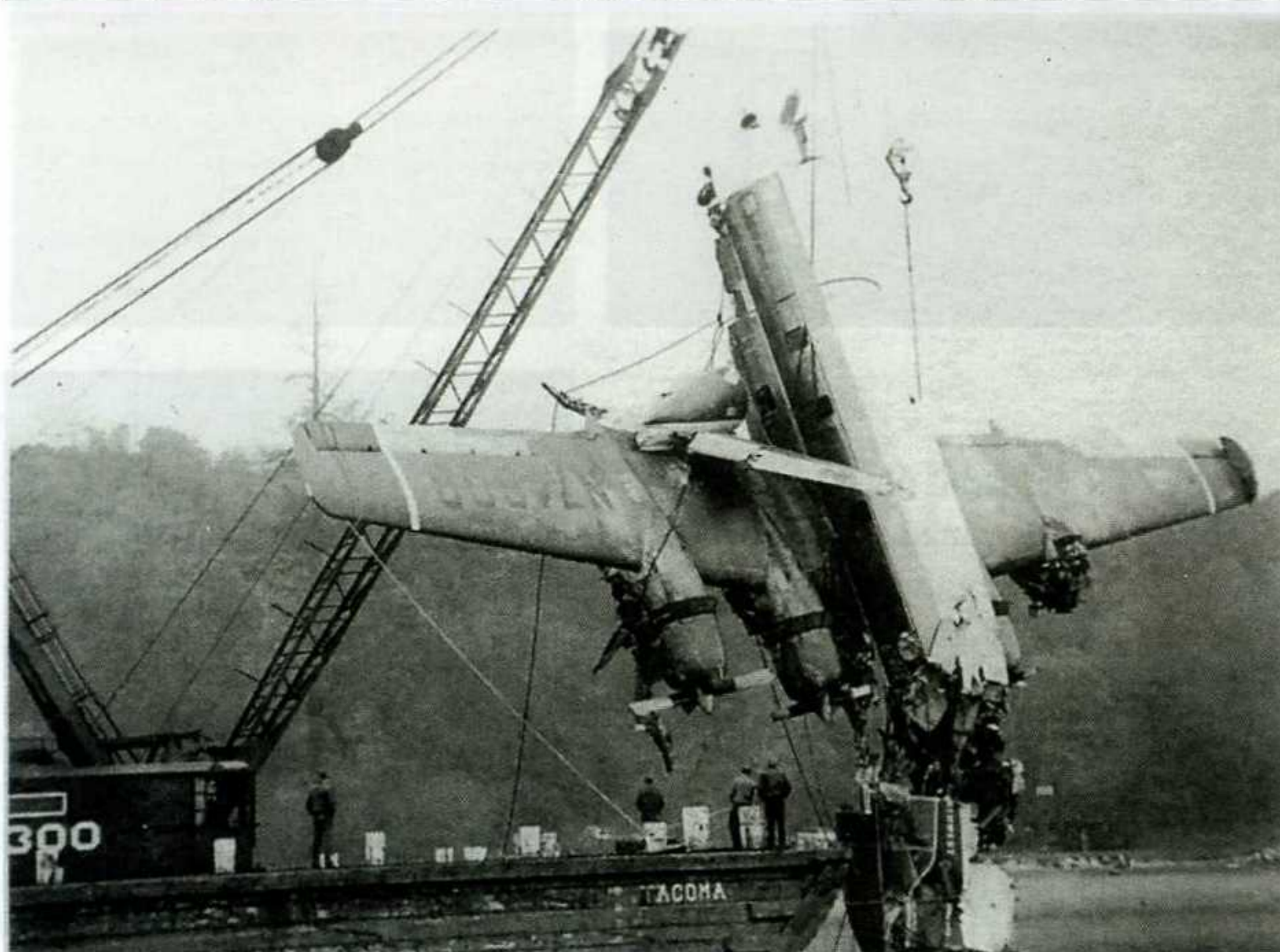
ABOVE: Foss 300 crane lifts the 60-ton plane after it was dragged into water of 45 ft. depth. Note the open engine cooling flaps. She was placed on a barge and towed to Tacoma by the tug Foss 18. Photo: Courtesy of Foss Maritime.
